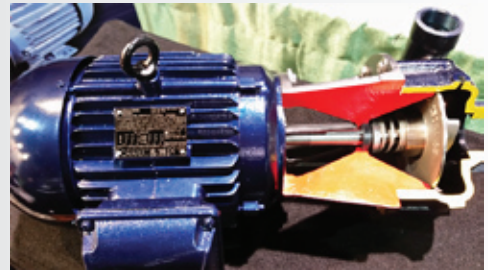
A work of art by Gary Smith...a Gusher V11019ah-se-a cutaway, specially engineered for dirty water service.
