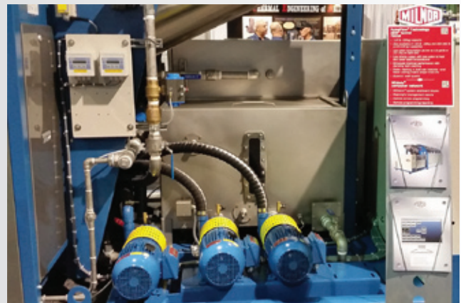
These three Gusher pumps are mounted on a tunnel drum commercial washing machine...featured at a Gusher customer's booth.
