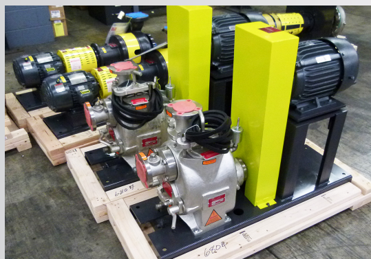
The Pumps are shipped with belts disengaged to insure the Customer goes through the proper testing process before use.
