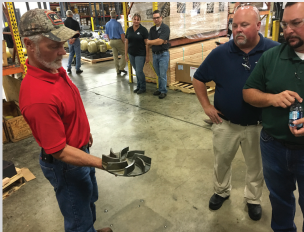
Tim Bowen describes the features of a Vortex Pump impeller.
