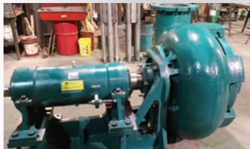
A demonstration of the Nagle Skimmer Pump, used for oil removal in Steel production and other industries.
