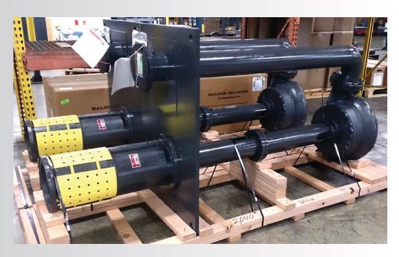
Mike Jones sends these...a couple of nice vertical pumps. These are Gusher V6X8 -15 - VSEL +47-CDM-A-DP, 73 7/8" long, rated at 1500 GPM at 43 TDH , driven by 60 HP at 1800 RPM motors, going into the Honda CAPT plant pumping coolant and chips back to a coolant filtration system
