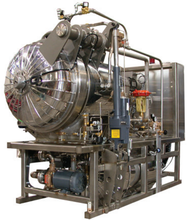
Jack Kirkwood reports a Gusher close coupled ANSI pump installation at ALLPAX Products. These pumps are being used in sterilization retorts for food processing industry and the application is superheated water.
