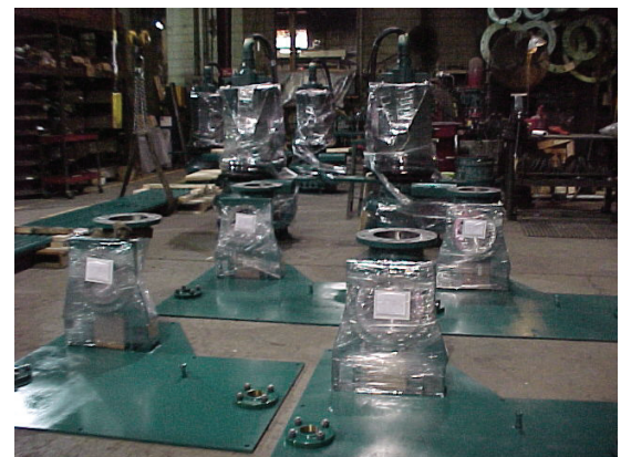
Bill Hein sends these photos of Nagle Submersible pumps with a quick-disconnect assembly being shipped to a Nucor Steel for handling steel scale.
