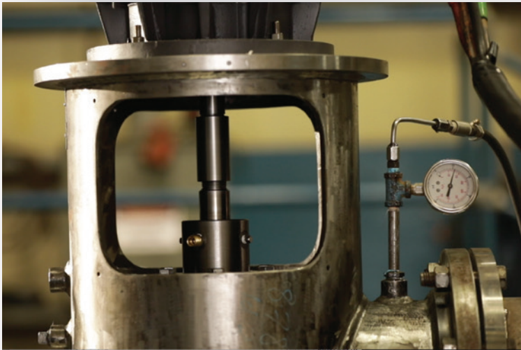
Running smoothly, at the expected at 1800 RPM...25 HP
