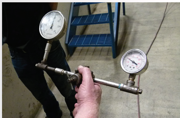
Joe created this custom made tool for checking gauge accuracy...AKA "The Hillbilly Guage Equalizer".
