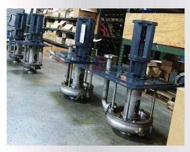
These finished Top Pull Outs are awaiting motors. Also sold by Great Lakes Pump and Supply, these operate at 15 Hp, 45 PSI, pumping 150 GPM.
