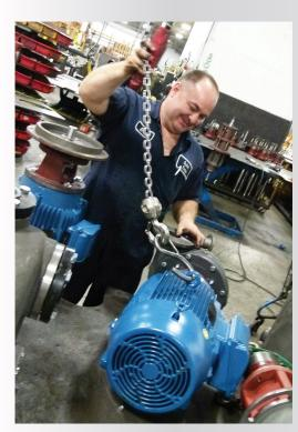
Shon Robinson handles a Close Coupled 7600 Horizontal, 25 HP, 3500 RPM pump.
