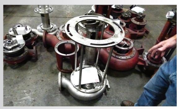
Assembly parts for a 4 x 6 x 13 Top Pull Out 7600
