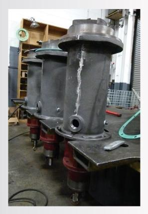
Shown here are Three 3 x 4 x 10B Enclosed Column Pumps ready for finishing..
