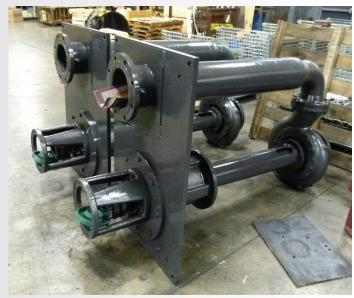
Tim Keetor shown here working on one of two Giants. These 7550 Vortex Pumps are 75 HP, 1600 GPM and designed foe an 88 inch immersion depth. These will be going back to the Dry Ridge facility for a customer witness test for a Great Lakes Pump and Supply customer.
