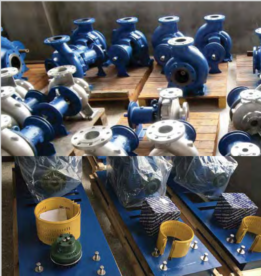
A large order of Gusher Shanghai manufactured Block DIN pumps ready for motor installation.
