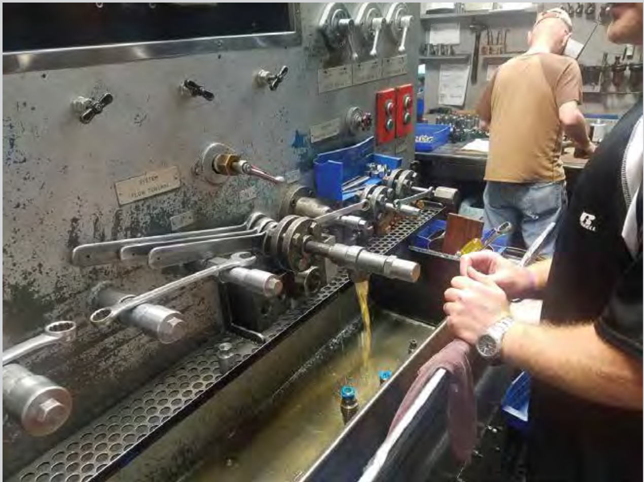
A Fulflo valve going through a quality control function test on this specially constructed test stand.
