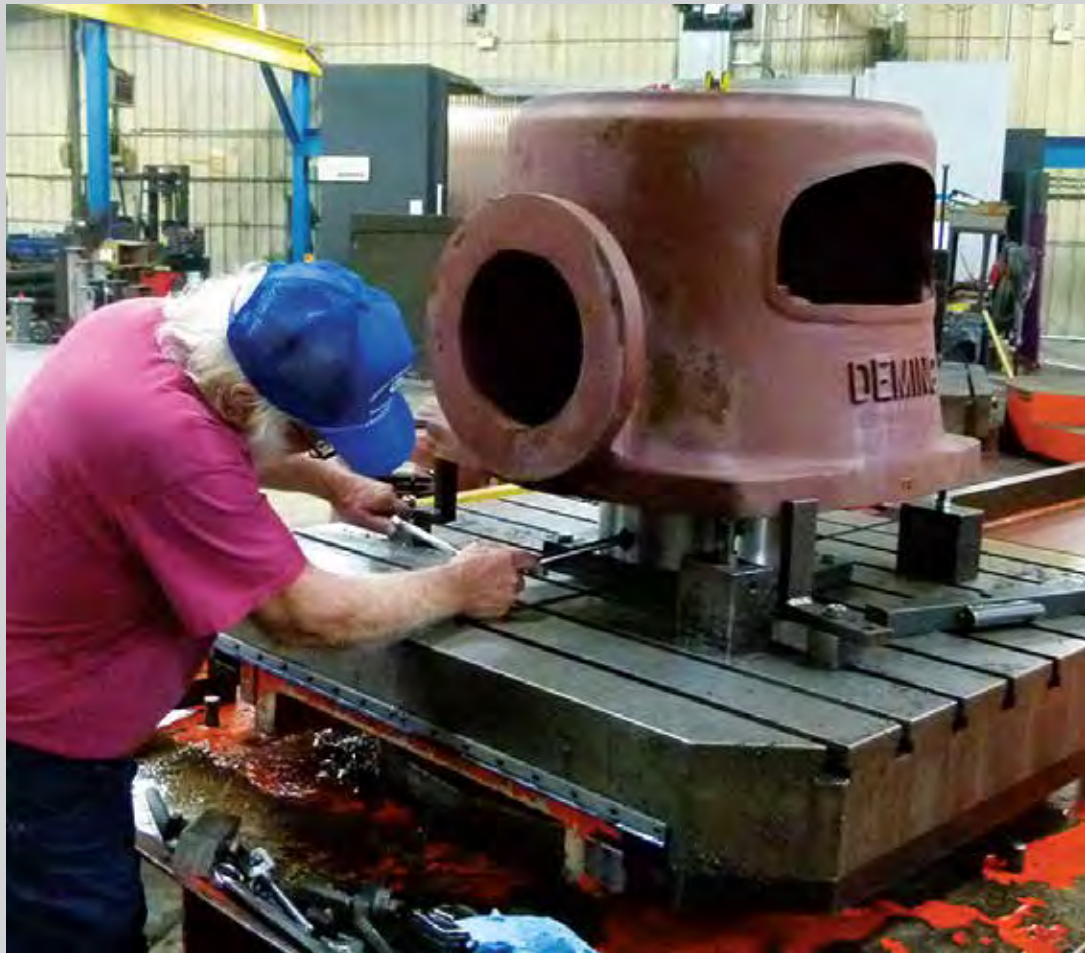
Milling a Deming head at the Gusher Dry Ridge location. Resources within Ruthman Companies are often shared to help complete projects.
