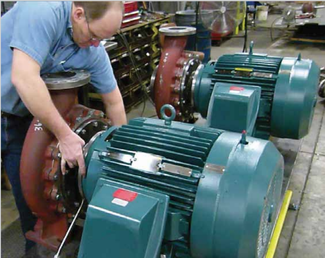
Assembly process of a DIN pump order at the Gusher Williamstown facility
