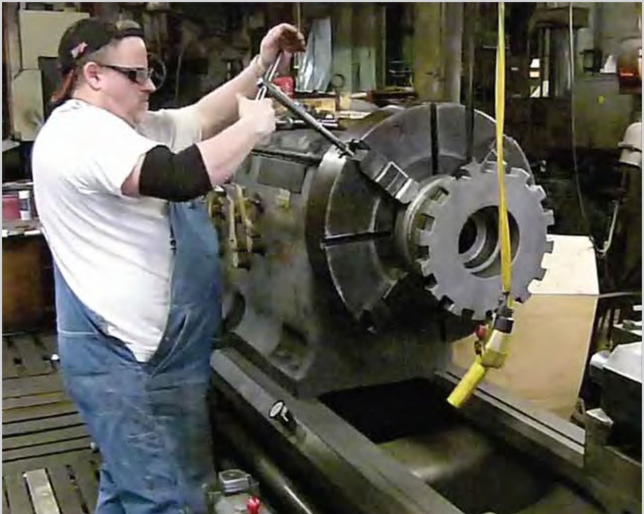
Getting ready to machine a Nagle thrust bearing housing in a lathe.
