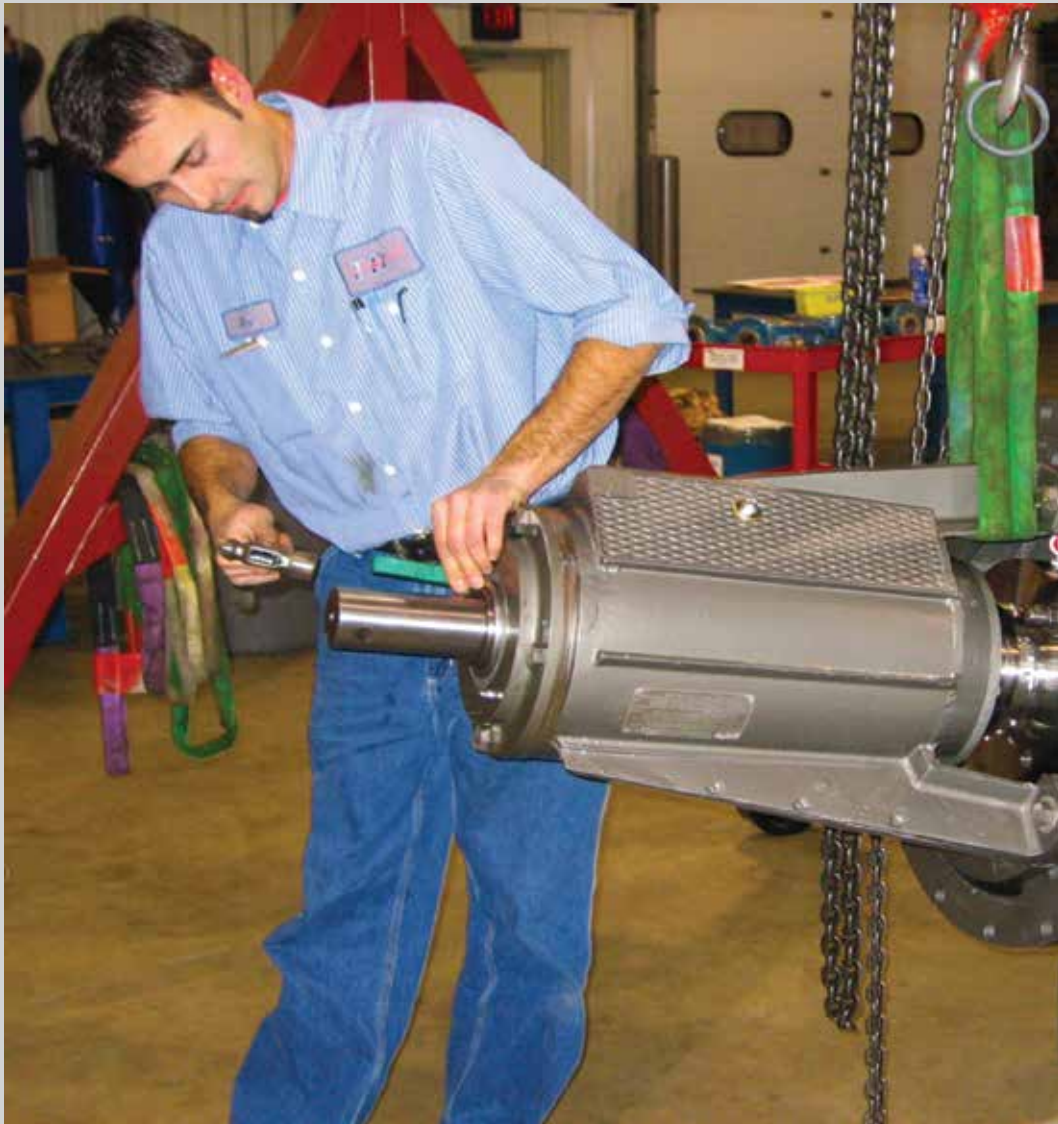
Setting the shaft on a pump at the Ruthmann Pumpen facility in Baesweiler Germany.
