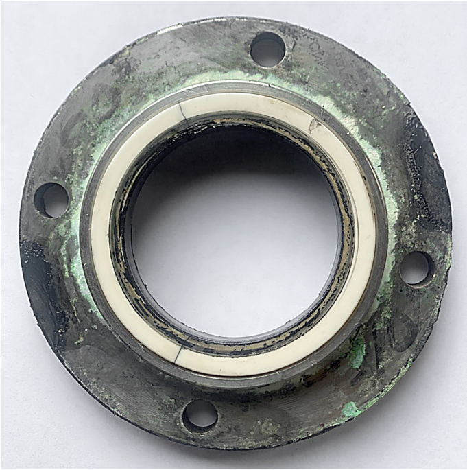
Figure 1 Failed mechanical seal exhibiting cracked seal faces and paint buildup
