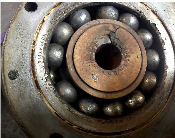
Figure 2. Failed thrust bearing, caused by excessive radial loading.
